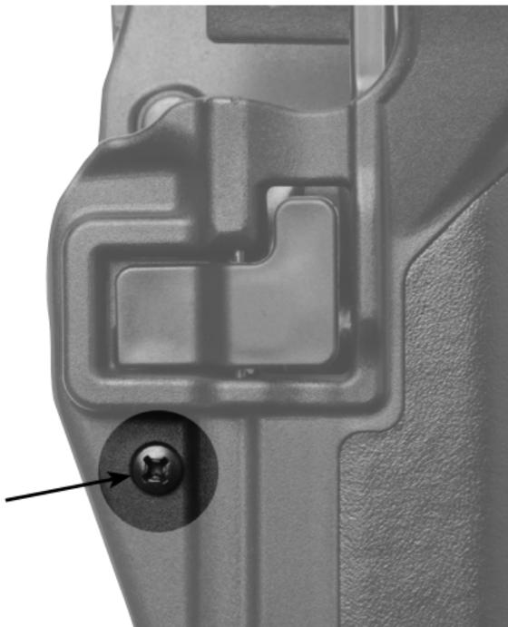
**NOTE:** Loosening the passive retention screw too far on Level 2 and 3 Duty Holsters will release the SERPA® rail adapter spring. If this occurs, simply place the spring back into position as depicted below and tighten the passive retention screw until there is a slight gap between the bottom of the screw and the surface of the holster body.
