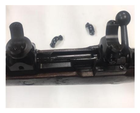
Ensure that the ring saddles (where the optic will lay) is free of debris or foreign material to include lubricant, grease, oil, etc. The optic can be placed into the rings
