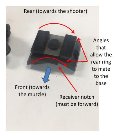
There are several ways to mount these bases and as mentioned, the bases can be soft soldered to the receiver in order to position them prior to drilling and tapping. One product that can be used is TIX soldier, it has a very low melting point (will melt and flow at 275 degrees) and has a good adhesion tinsel strength.
