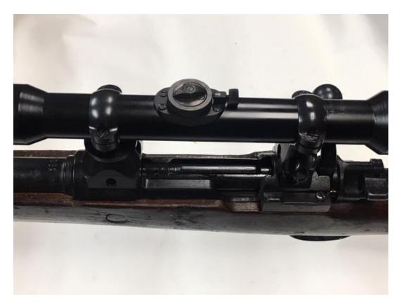
Note: Ensure that the rear locking lever is tight to lock the ring into position on the base.
