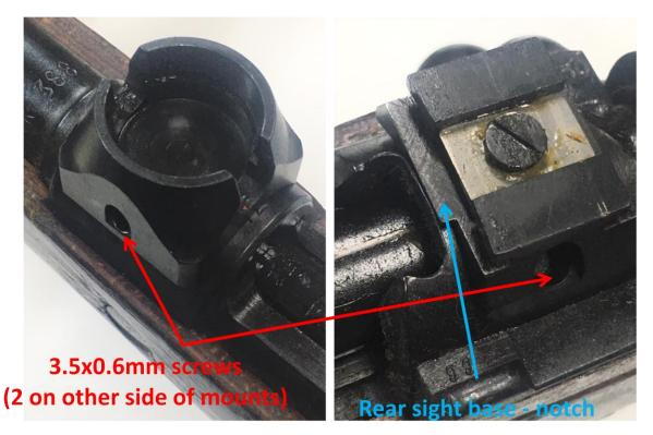
NOTE: The rear bas MUST be put on correctly or the optic will not be able to be installed or removed. The base has an angle cut into the front and back of it (relative to the receiver, the angle is slightly circular).
