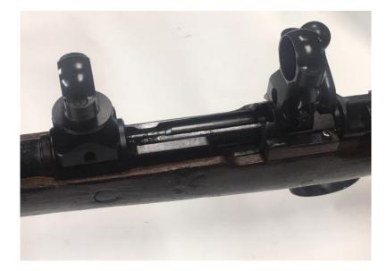
After the rings have been installed, the ring caps can be removed
