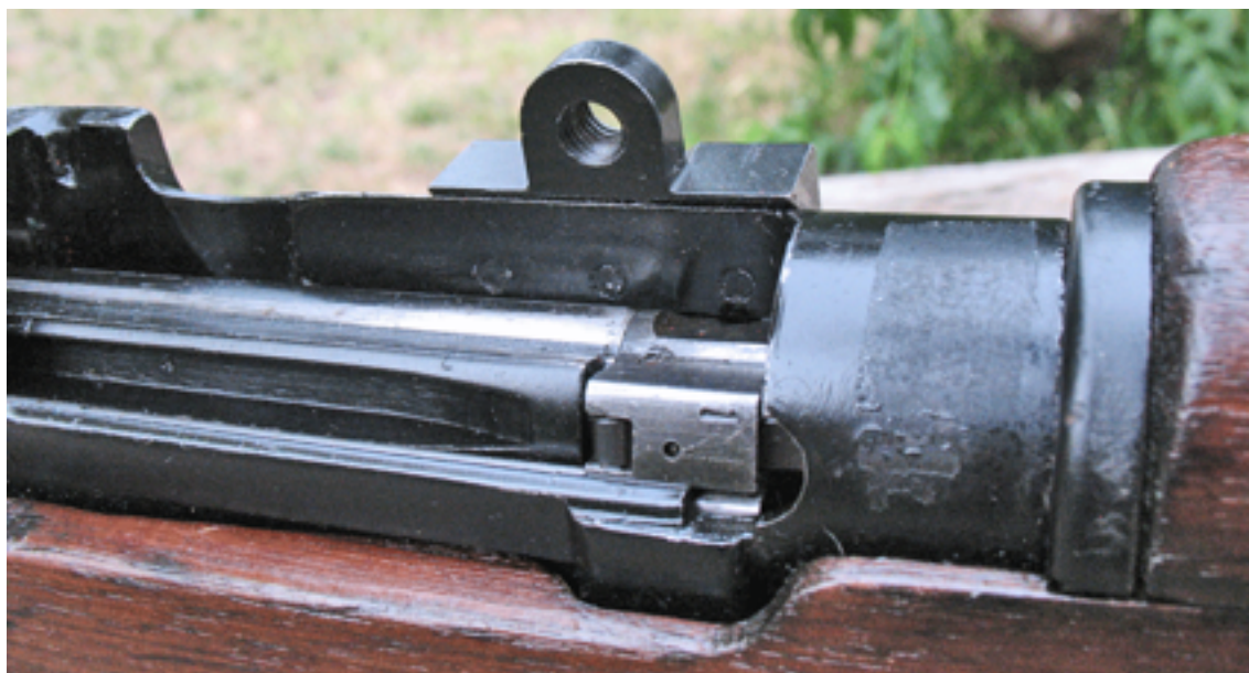
Fig. 10 - Front pad in situ - right hand side front showing mounting screws protruding through sidewall of rifle. Note the levels of the rifle sidewall and the lip of the pad.
