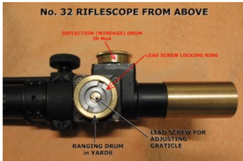
Fig. 4. - No. 32 riflescope showing adjustment mechanism.
