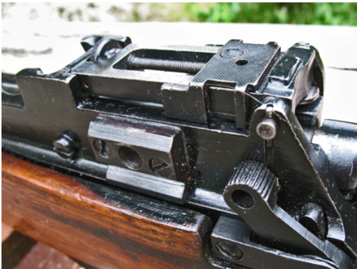
Fig. 11 - Rear pad in situ. Note the lower moulding which seems to be designed to allow the pad to sit on a protruding ledge of the sidewall of the No. 4 rifle.
