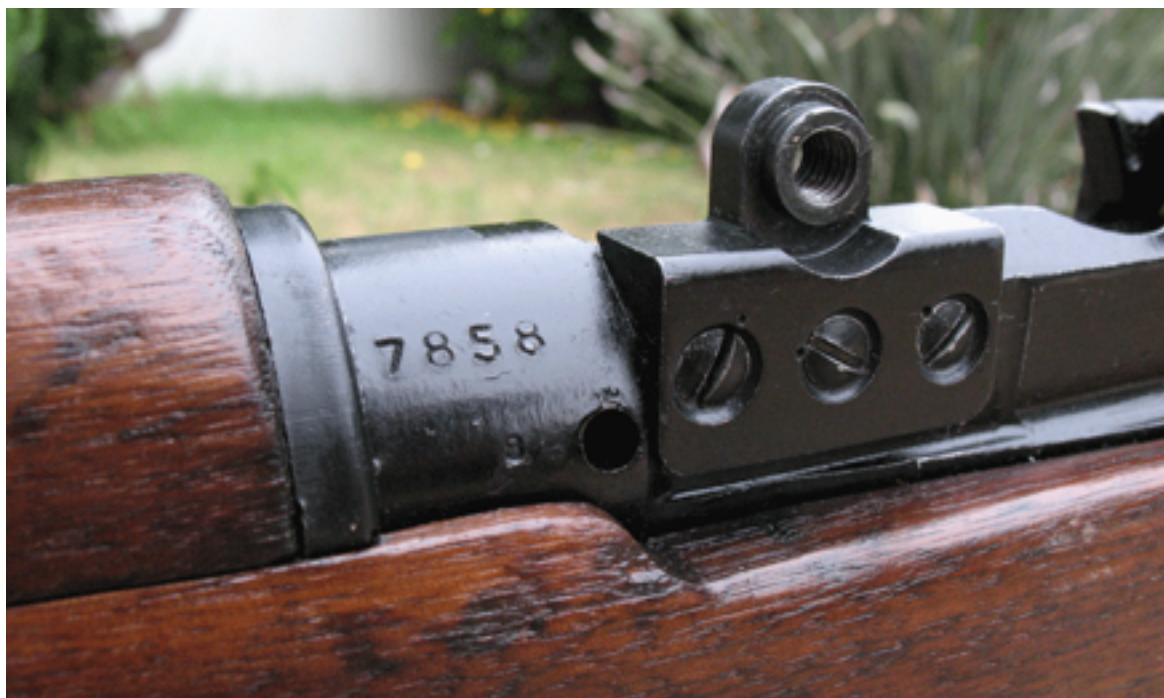
Fig. 9 - Front pad in situ - left hand side front showing mounting screws.
