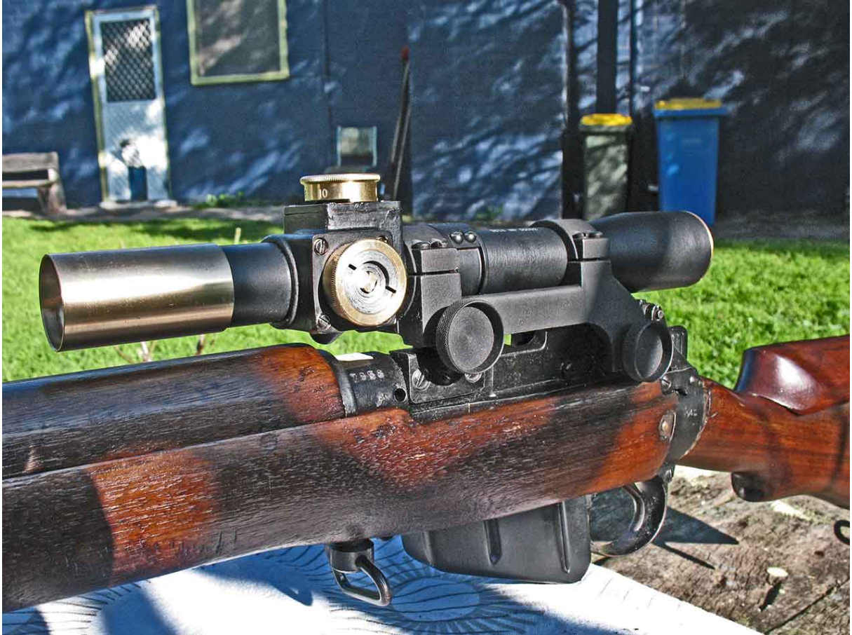
Fig. 1 – RSM replica of the famous British No32 sniper scope mounted in another replica of the special bracket (mounts) attached via the pads (bases) to the sidewall of a No4 Mk1 rifle.
