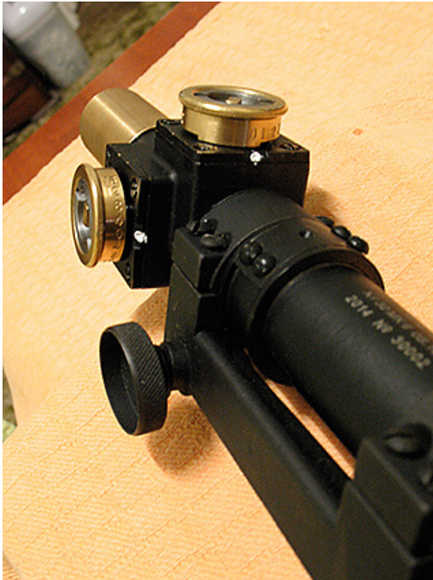
Fig. 5 – Range and deflection drums on the No32 scope (from behind).
