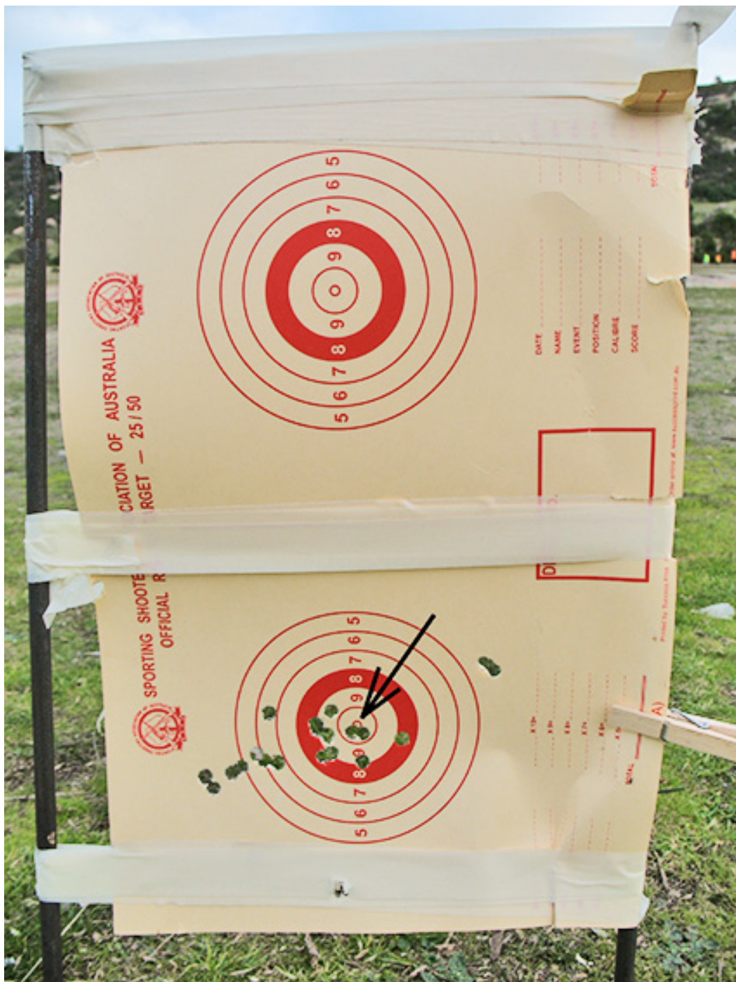
Fig. 7 – Zeroing at 25 yards. The 3 bullet holes on the middle circle (arrow) are the final adjustment after getting used to how the drums shifted the graticule.
