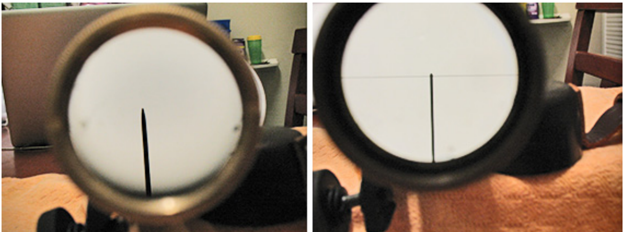
Fig. 8 – Graticule on the prototype scope (left) compared to the correct graticle from author's original scope (right).
